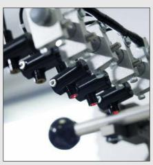
Accurate positioning with the help of the 5 position lamps
