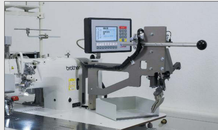
The swivel-out folding station enables easy access for set-up and service work
