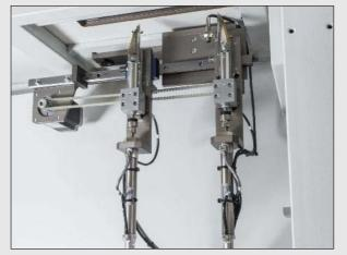
Cutter block with stepper motor drive
