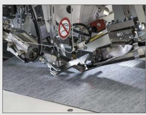
Pneumatic scissors for cutting off the endless zipper
