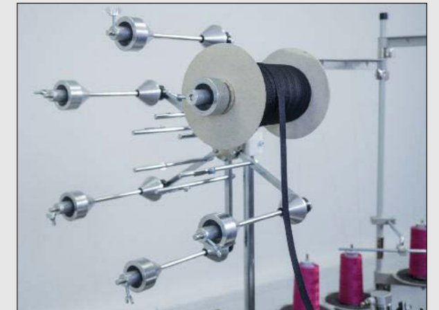
Bobbin holder and magazine function
