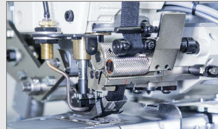
Exact tape guide to the sewing base
