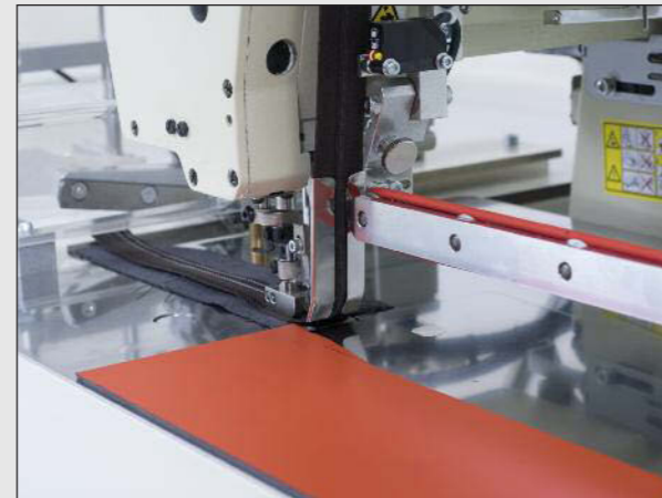
Machine stencil and zipper guide ensure consistent seam quality and guarantee the optimal seam result
