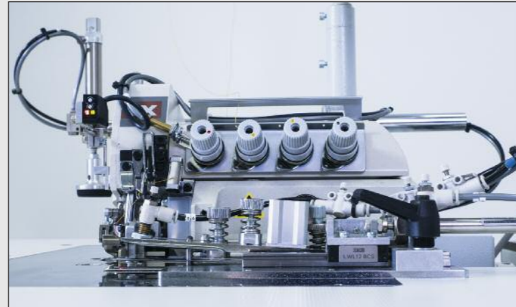
The accurately adjustable contour guide ensures consistent seam widths over the entire length of the seam
